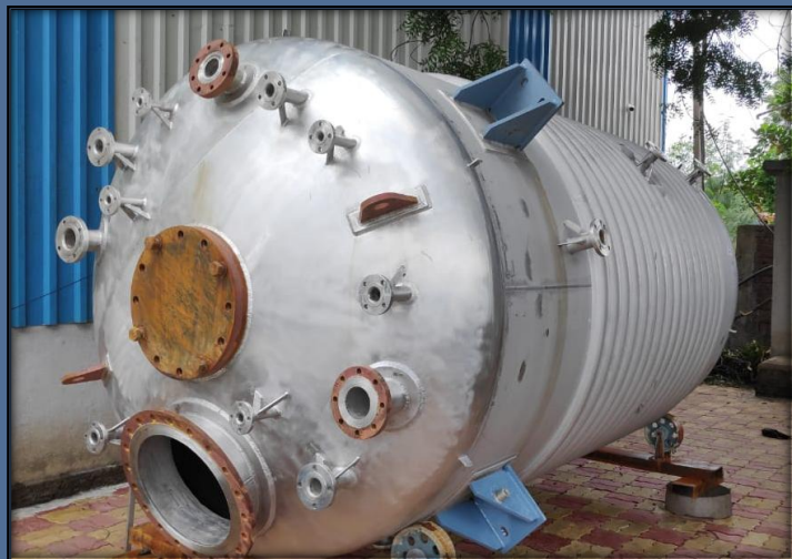
Limpet Coil Reactor
