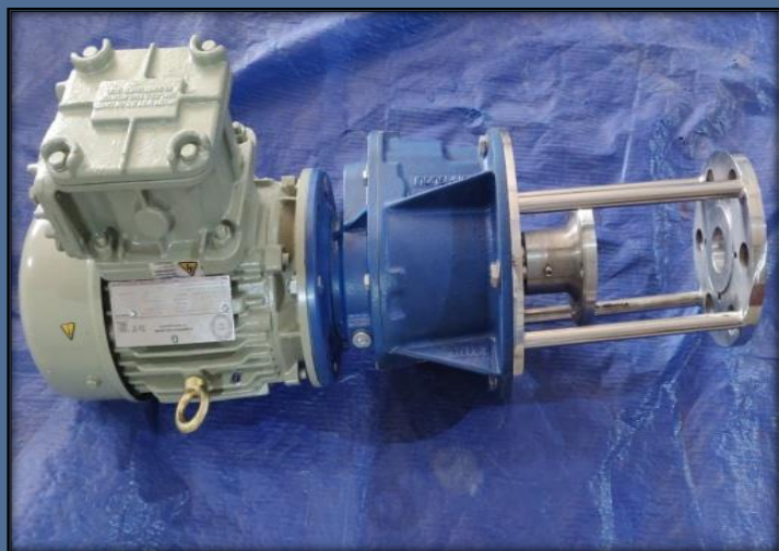
Anchor Agitator Assembly (Pharma Application)
