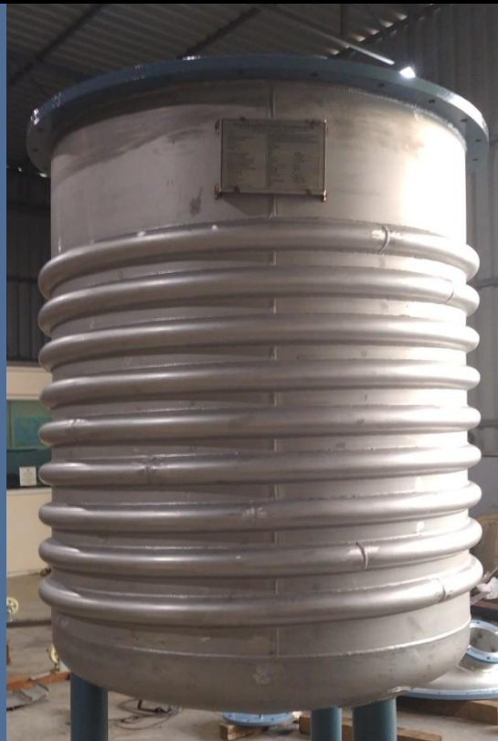
Reactor with Body flange & Limpet Coil
